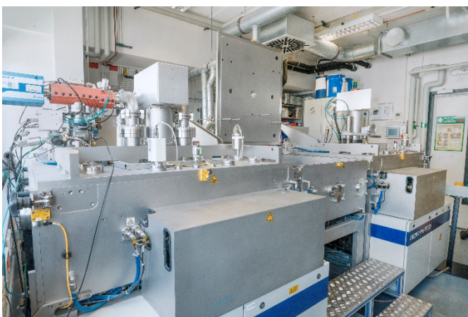
Picture 2: Chemical vapor deposition (CVD) coating plant used to produce functionalized textiles.
